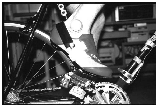
Figure 6 Kinetic analysis with a 6 load pedal dynamometer.
